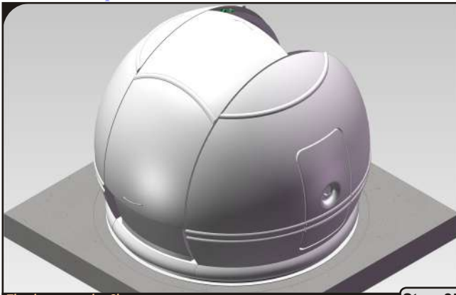
The dome panels - Shutter
