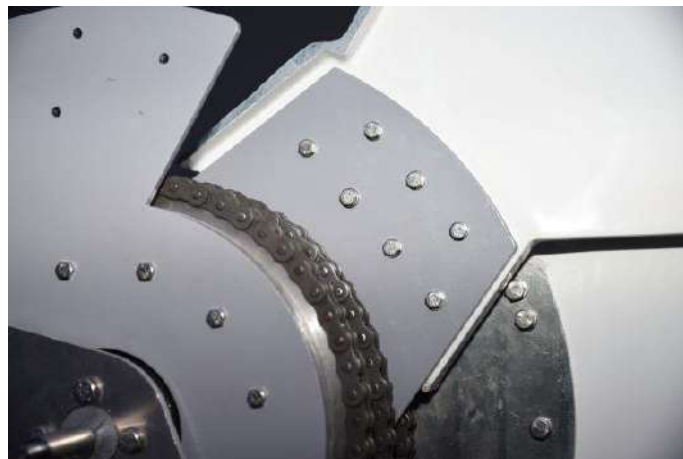
Figure. 48 – Screw connections of shutter No. 2
