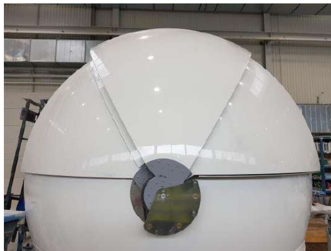
Figure. 56 – observatory with shutters installed in closed position
