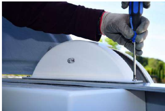
Figure. 58 – installation of the gear inner cover
